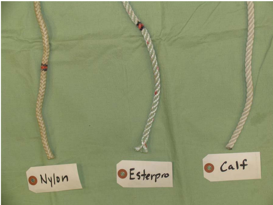
Figure 2. Buoy line types used in this study: diamond-braided (#8) nylon; Esterpro™ (#8 medium lay) polysteel filaments/polyester; polypropylene with wire core (#8.75) calf.
