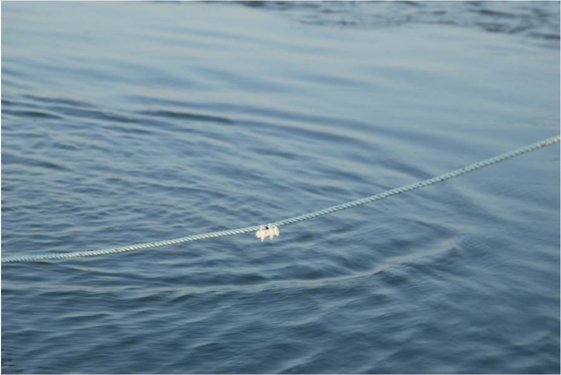
Figure 3. Example of attachment of DSTmilli logger with cable tie on Esterpro buoy line.
