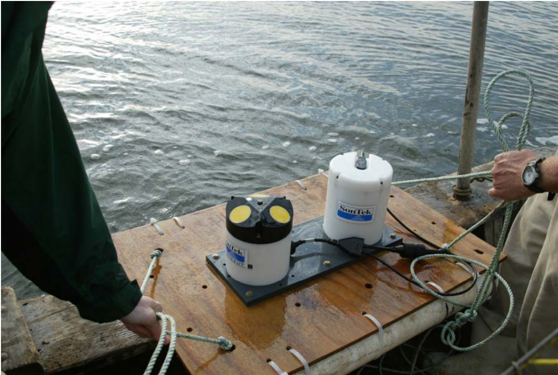
Figure 4. Configuration of Argonaut XR current velocity meter. The white cylinder on the right is the battery.
