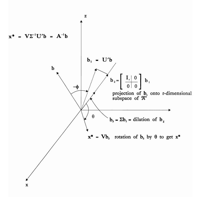
Figure 3. Geometric interpretation of least squares solution in terms of singular value decomposition.
