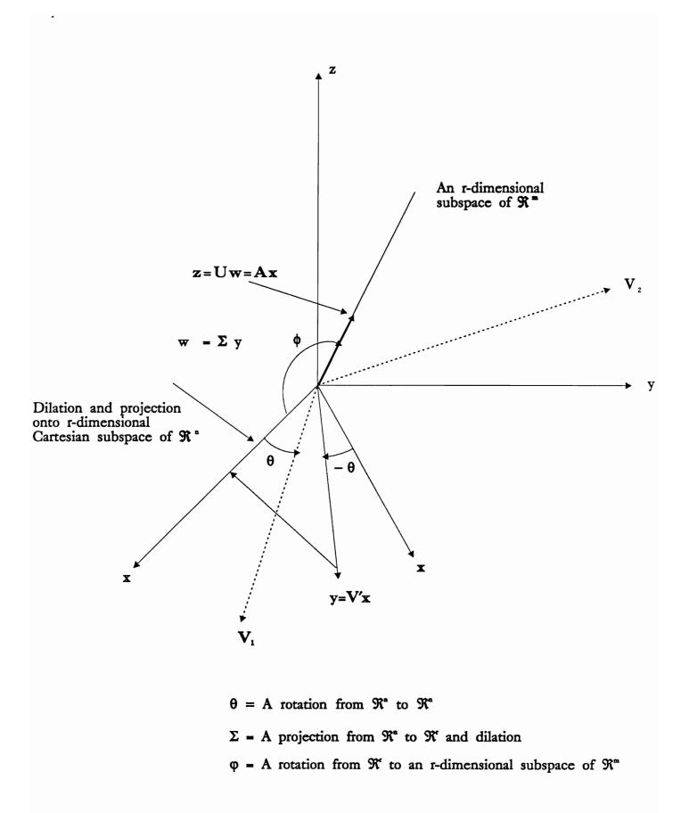
Figure 2. Geometric interpretation of singular value decomposition for r=1, n=2, and m=3.
