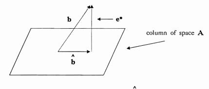
Figure 1: Orthogonal decomposition of **b** into **b** and **e**\*
