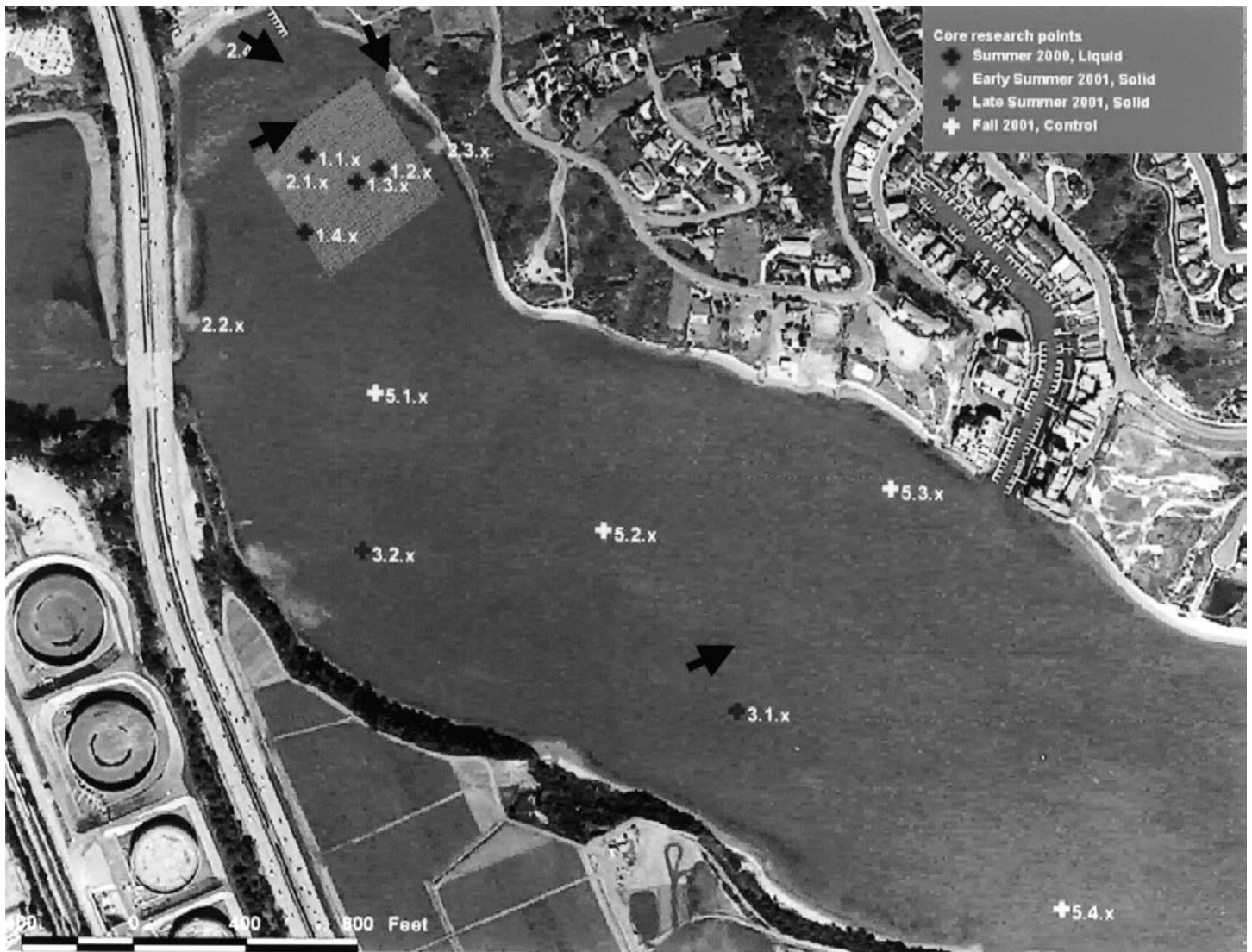
Figure 2. Map showing locations in the inner basin at Agua Hedionda Lagoon (Carlsbad, CA) where core samples were taken to assess efficacy of eradication treatments in December 2001. Legend indicates treatment date and type of treatment. Arrows show locations where second set of cores were taken in August, 2002.
