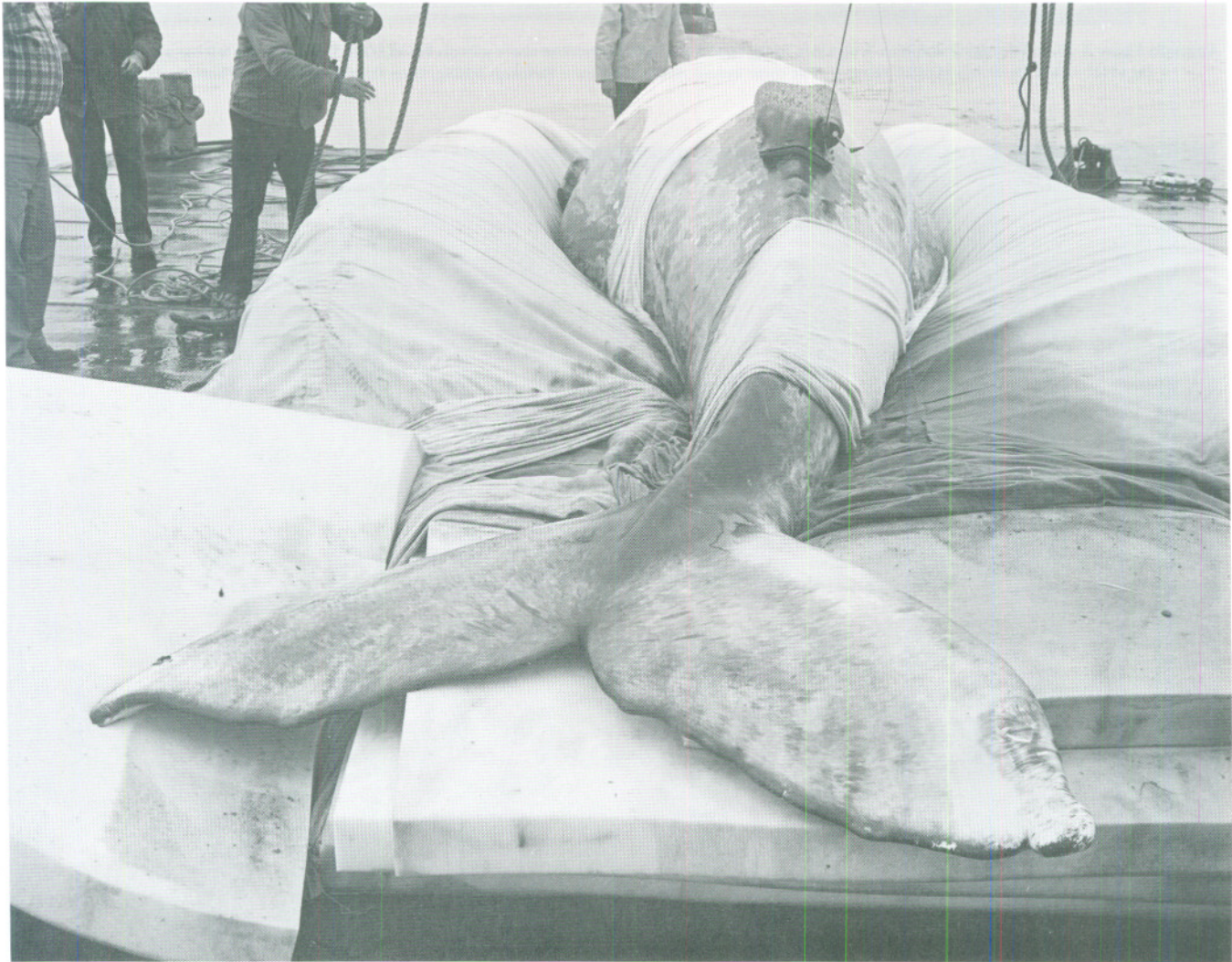
Appendix Figure A-15.—A radio transmitter package surgically attached to the dorsal ridge of a California gray whale. This yearling animal, captive for most of the first year of its life, was released into the ocean off San Diego, Calif., in March 1972 and was subsequently tracked from shipboard and aircraft for over 30 days. The sensor-transmitter package, shown in detail ( top), was designed to measure the maximum depth of the animal's dive and the water temperature at that depth. (Photos by S. Leatherwood.)
