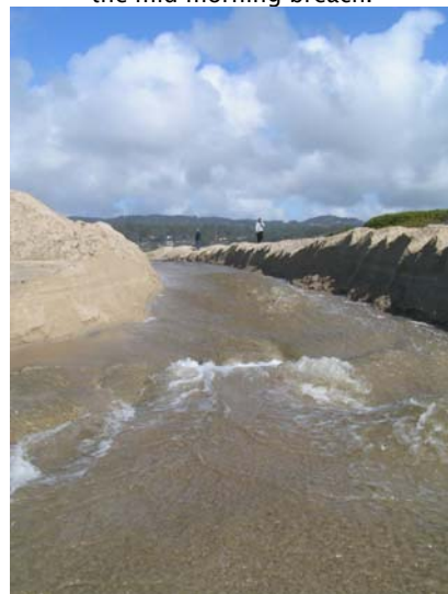
g. At 11:00, flows increased and small rapids formed but the stage remained at 2.6 m.
