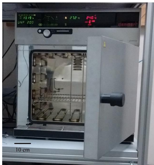
Fig. 6.7 – Photograph of the Memmert Furnace; temperature controlled environment from 5 °C above ambient to ~ 300 °C.
