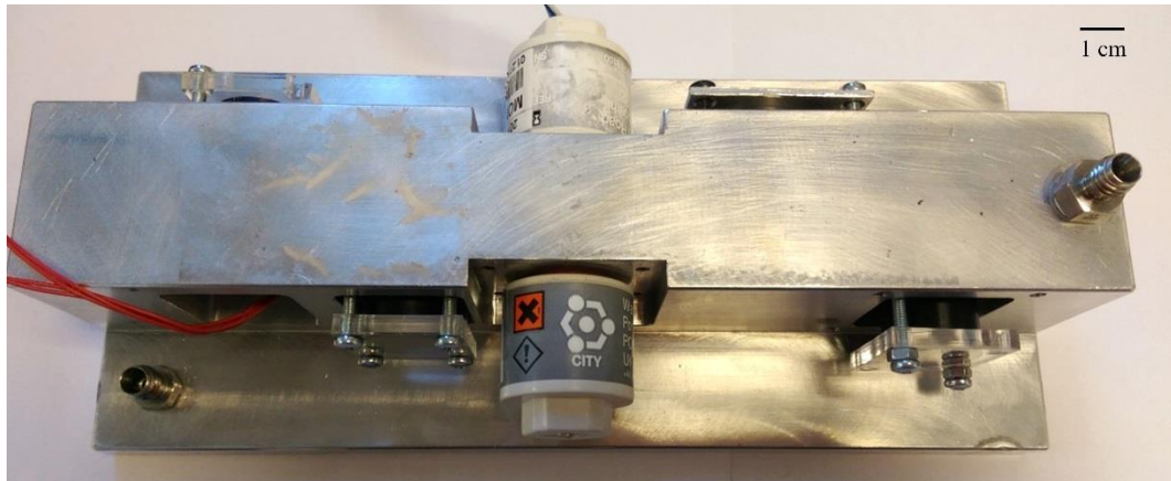
Fig. 7.6 – Photograph of the aluminium chamber to house O_2 sensors for the experiments, with a temperature and humidity sensor fitted to measure environmental conditions.
