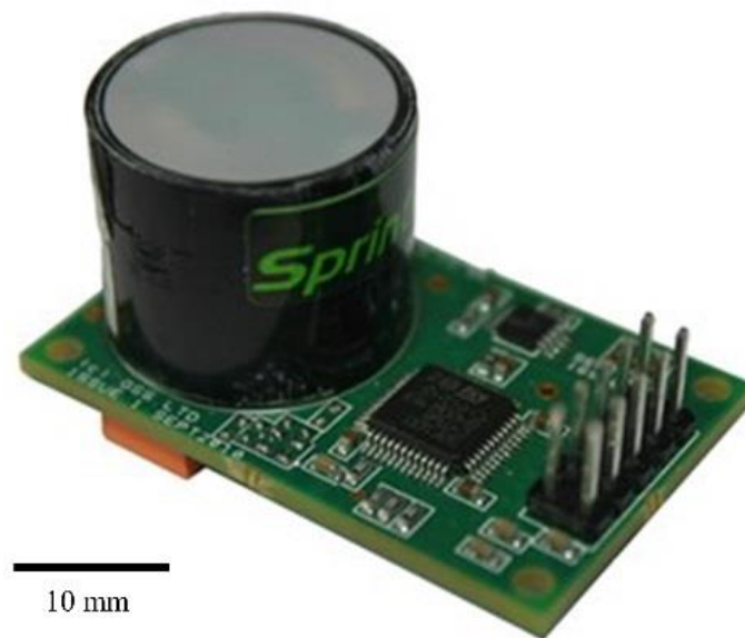
Fig. 3.14 – Commercial NDIR sensor, 20 mm diameter sensor offers CO 2 detection up to 100 %, given the range of models available [98].
