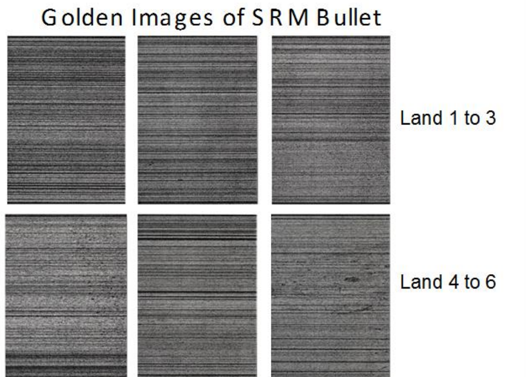
Fig.2-14. The “Golden Image” of six Land Engraved Areas (LEA) of the SRM 2460 Standard Bullet.
