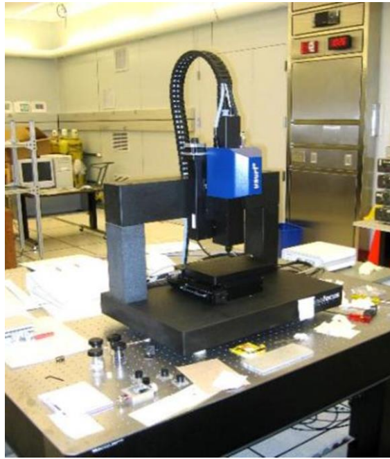
Fig.2-12. A Nanofocus confocal microscope was used for 3D measurements of SRM Cartridge Cases.
