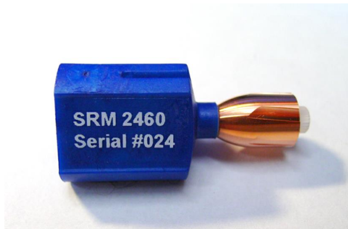
Fig.2-6. A NIST SRM 2460 Standard Bullet mounted on a blue stub for initial setup on a microscope.
