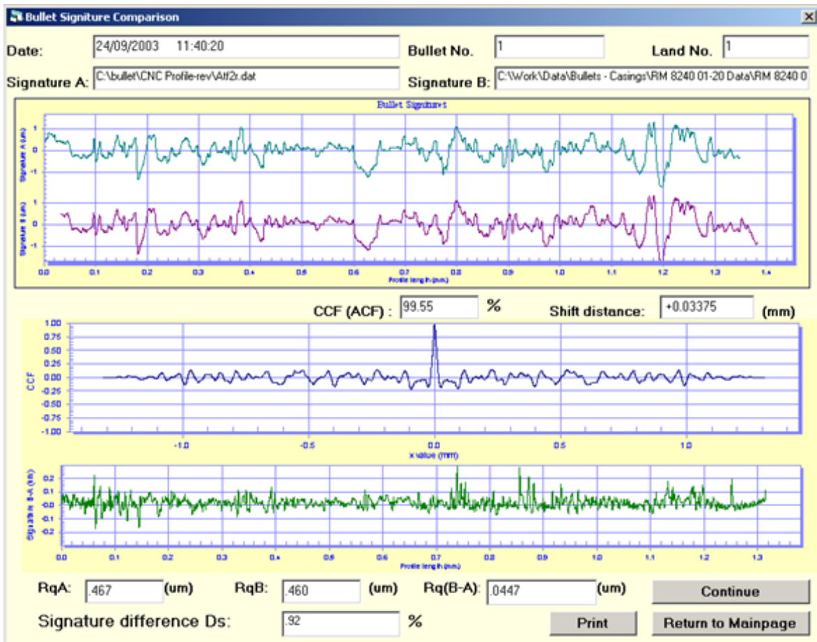
Fig.2-10. User screen for bullet signature measurement between the land 1 of SRM 2460-001 Standard Bullet (Signature B, as shown on the second profile from the top) and the virtual standard (Signature A, as shown on the top). The cross-correlation function CCF_{\max} = 99.55\% , the signature difference D_s = 0.92\% . The units of the top and bottom vertical scales are \mu\text{m} . The unites of the lateral scales are mm.
