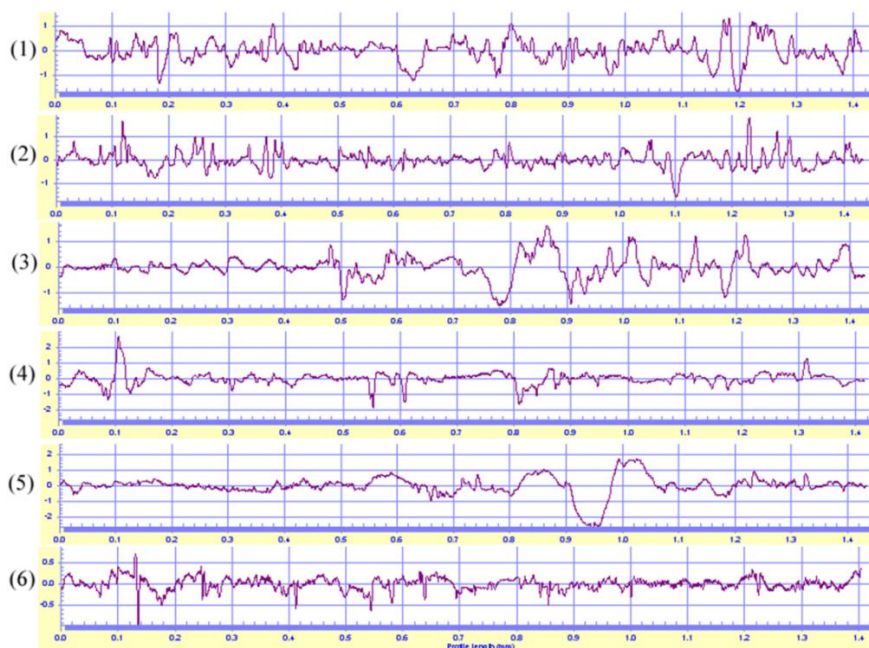
Fig.2-3. The virtual bullet signature standard consists of six digitized bullet profile signatures measured by a stylus instrument on six master bullets fired at the ATF and FBI. The virtual standard profiles shown above are modified profiles after curvature removal and Gaussian filtering with a short-wavelength cutoff of \lambda_s = 0.0025 mm and a long wavelength cutoff of \lambda_c = 0.25 mm [5]. The vertical scale is in \mu\text{m} ; the horizontal scale is in mm.
