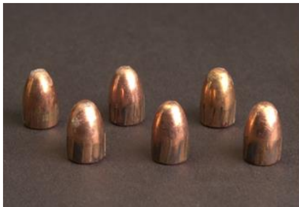
Fig.2-2. Six master bullets from ATF (top row) and FBI (bottom row), each of which was traced on a selected land engraved area. The six digitized bullet signatures were stored in a computer as the virtual bullet signature standard.
