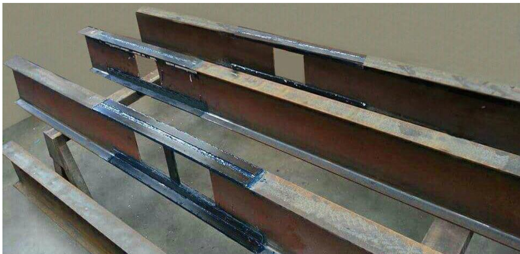
(b) Upturned specimens during curing of adhesive
