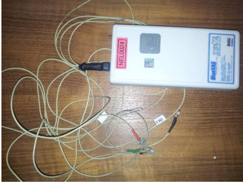
Figure 2.8: Example of EEG portable system to record EEG with 2 channels system plus ground and reference channels.
