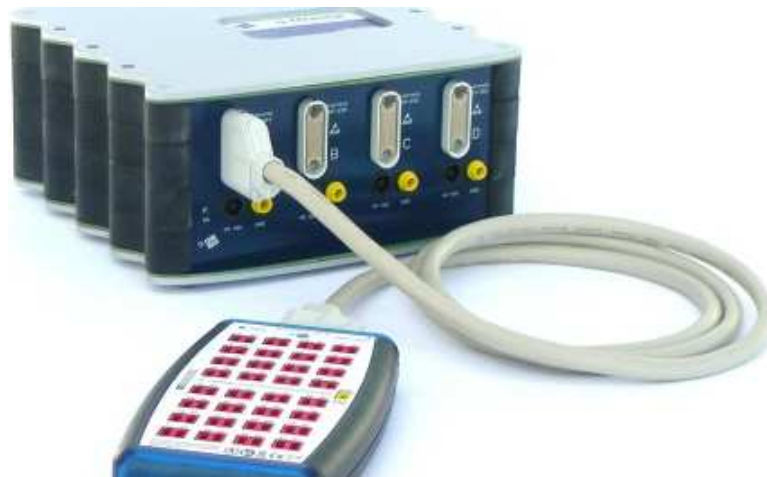
Figure 2.9: Figure (A) shows a g.tec g.GAMMAsys with 64 electrodes applied and (B) shows a g.tec g.HIamp amplifier [67]. The cap and amplifier are interconnected and linked via a USB to a computer.
