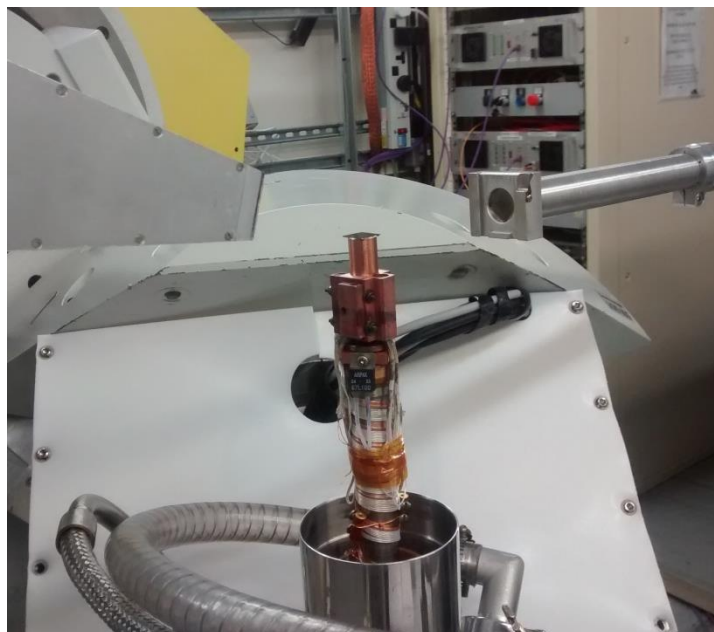
Figure 3-12 A GeSn/Ge/Si sample mounted on copper stub via silver paste and mounted onto the high temperature cryostat sample cradle. To the right is the X-ray beam source, to the left is the flight tube to the detector.
