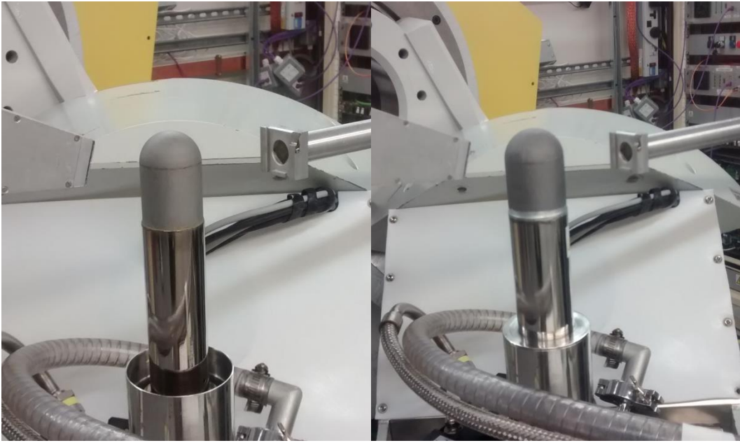
Figure 3-13 The high temperature cryostat with (left) the inner cryogen shield mounted, to contain the cryogen (right) the outer vacuum shield mounted, which is used to maintain a vacuum for thermal insulation.
