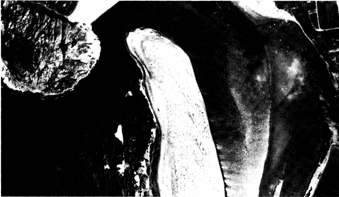
BY 1938, A REVETMENT AND SUBSEQUENT ACCRETION OF SAND BEHIND IT FINALLY CLOSED THE OLD NORTH CHANNEL. NOTE THE SHOALING ALONG THE FRONT OF THE TOWN OF MORRO BAY. (PHOTO (ABOUT 1938) - FROM WIEGAL, 1967)
