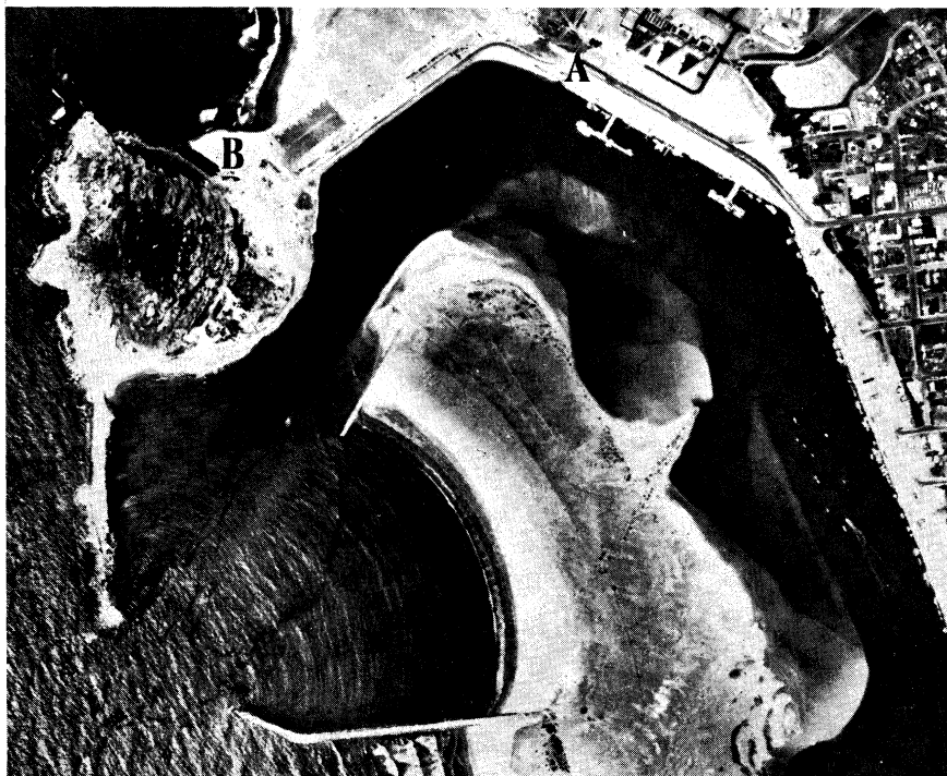
BY 1946 THE SOUTH AND MORRO ROCK BREAKWATERS WERE CONSTRUCTED AND BY 1956 THE NAVIGATION CHANNELS DREDGED, BY THE U. S. ARMY CORPS OF ENGINEERS, FORMING THE PRESENT ENTRANCE TO MORRO BAY. NOTE THE PACIFIC GAS AND ELECTRIC CO. PLANT, THE WATER INTAKE AREA (A) AND THE WATER DISCHARGE CANAL (B). (PHOTO BY THE U. S. GEOLOGICAL SURVEY - JUNE, 1963)
