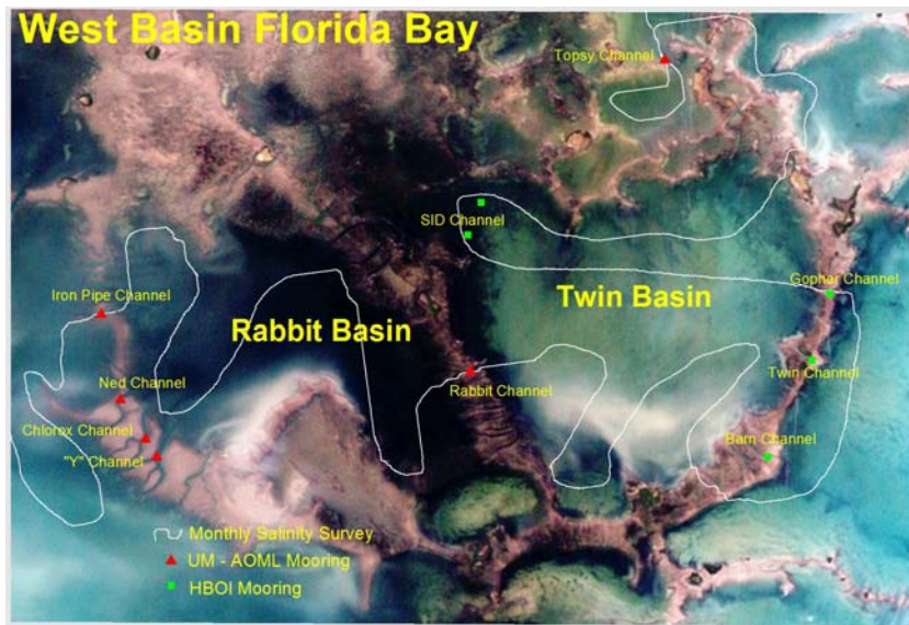
Fig. 1. Location of Rabbit Key and Twin Key basins within the western sub-region of Florida Bay. Current and salinity time series were made during wet (Jun to Nov 2004) and dry (Dec 2004 to Jun 2005) seasons in channels connecting the basins to surrounding regions. Mooring locations are shown with solid triangles and squares. Shown with solid line is the vessel track of the bi-weekly salinity surveys.
