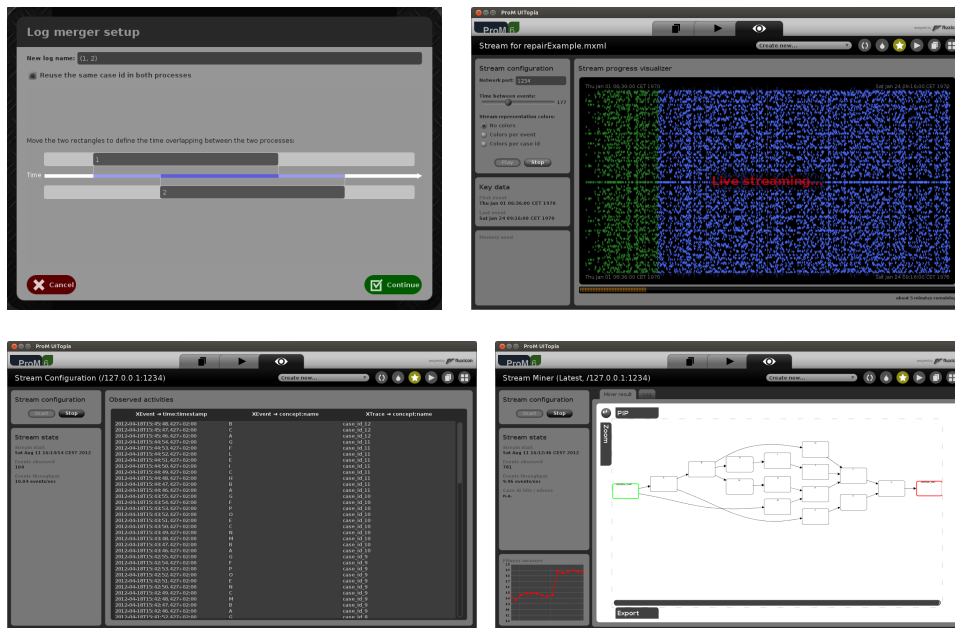
Figure 10.7. Screenshots of four implemented ProM plugins. The first image (top left) shows the logs merger (it is possible to define the overlap level of the two logs); the second image (top right) represents the log streamer, the bottom left image is the stream tester and the image at the bottom right shows the Online HM.
