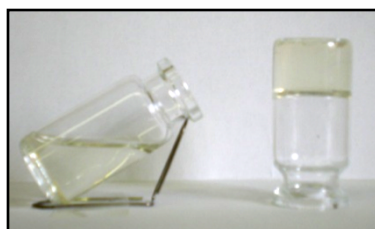
Fig.19 The clear sol (on the left) and the “tube inversion test” showing gel formation (on the right).
