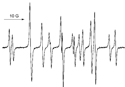
Figure 11 EPR spectrum of BTBN at 298 K recorded in water in the presence of CB7 7.0 mM.
