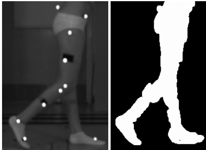
Fig. 6-2. Sample image and its segmentation output. As can be seen, complex background did not diminish the performance of the segmentation algorithm.
