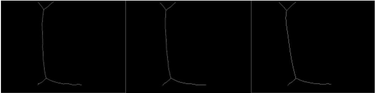
Fig. 4-6. Skeletonized outputs of Fig. 4-1 after MAT algorithm was applied.
