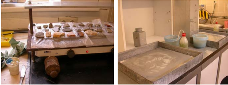
Fig.13-14 Heating table for the hardening of the resin and the equipment for the thinning procedure through abrasive powder of different granulometry (ELTE University laboratory in Budapest).
