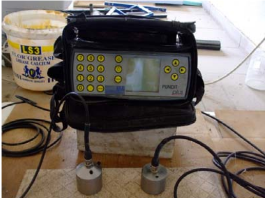
Fig.17-18 The equipments for ultrasound resistance and compressive strength tests
