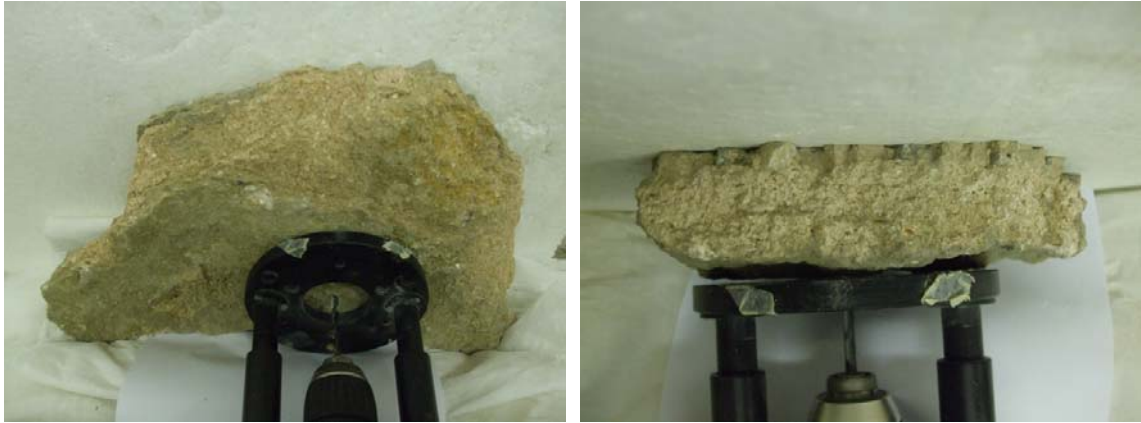
Fig.50-51 Two moments of the drilling test.
