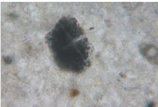
Fig.42-43 From the same mortar, on the right side picture it is visible a pozzolanic nucleus (magnification 10x, one N). On the left side picture it is visible a grain of Portland cement in bottom left and a dark pozzolanic nucleus at the top right (magnification 25x, one N).
