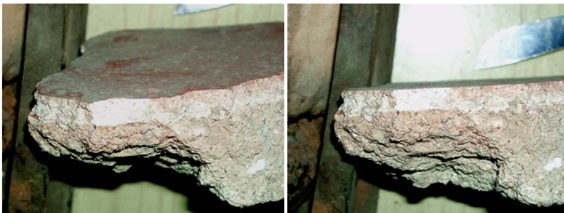
Fig.52 a) and b) The two different layers composing the structure of a mural painting fragment.
