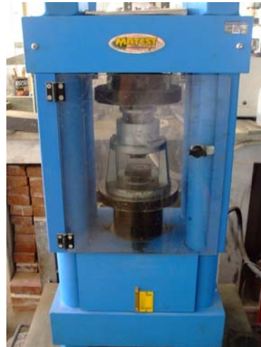
Fig.17-18 The equipments for ultrasound resistance and compressive strength tests
