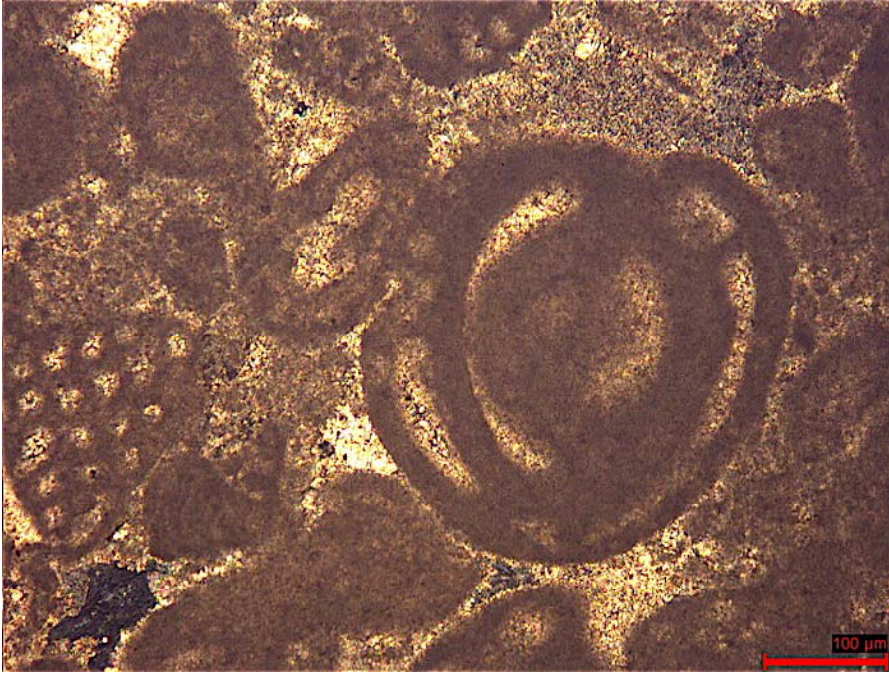
Fig.22 Detail of sample HUNVMEC4-3: Nagyharsány villa's walls. Biosparite with a big Miliolidae.
