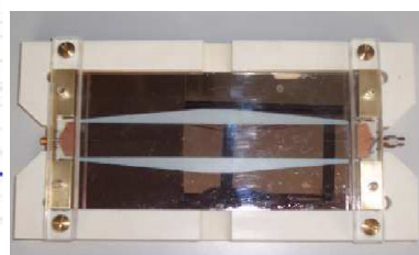
Fig. 12: Coplanar Wave Guide. Fig. 12a: Scheme of the CPW; Fig. 12b: Pictures of the set up used in the experiments.
