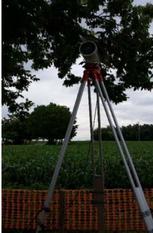
Scintillometer (transmitter left-receiver right) Eddy Covariance
