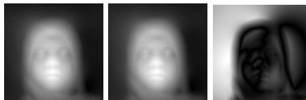
Fig. 4. Reconstructed surfaces using the proposed method with unknown illumination on the right and the ground truth on the left under different view points for the first dataset.
