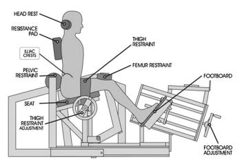
Fig. 3. MedX lumbar extension machine, showing restraint system.
