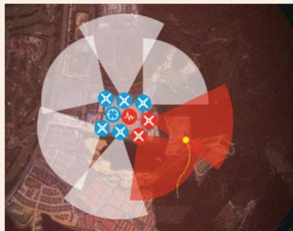
Figure 13: The technology has the ability to identify the make, model and capacity of the drone. The drone is visible as a yellow dot with a tail showing the path, which has flagged on the detection software in the red zones [59].
