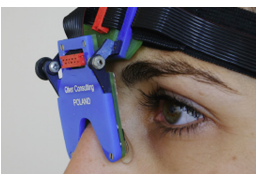
Figure 2.10: An example direct infrared oculography system: the Saccadometer by Ober Consulting.
