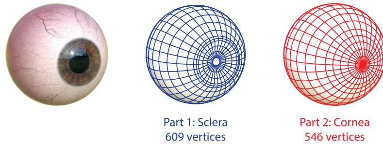
Figure 3.3: The two-part eyeball model that I used in each dynamic eye region model. Left: the full render. Middle, blue: the inner sclera part that uses a purely diffuse material. Right, red: the outer part that is a little bigger than the inner part, contains the corneal bulge, and is transparent and reflective.
