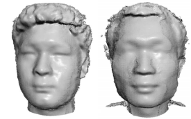
Figure 4.4: Raw scan data used in FW. Note how eye details have been smoothed out.
