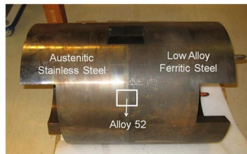
Fig. 1. Dissimilar metal weld mock-up (MC1) outer radius = 352mm, thickness = 40 mm
