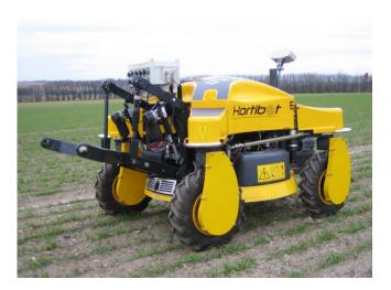
Figure 2. Hortibot field robot
