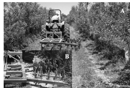
Fig. 1. (A) Modified notch disk tiller for the implementation and maintenance of the Swiss sandwich system (SSS) tilled strip. (B) Modification in the disk setup for the notch disk tiller.
