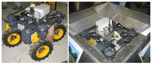
Figure 2. Left – The remotely controlled mobile unit. Right – The remotely controlled mobile unit within the pyramidal feeder construction (see also figure 3 right)
