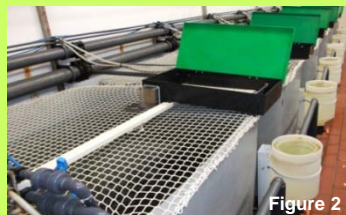
Growth performance was measured using a recirculation system consisting of 12 square formed fiber glass tanks and feeding each diet in duplicate for 9 weeks, from an initial weight of 60 g to a final weight of about 200 g (Figure 2).
