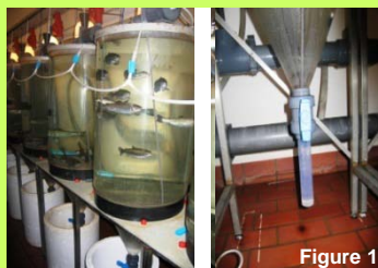
Digestibility of dietary nutrients was measured directly using a modified, flow through Guelph System consisting of 18 tanks, and feeding each diet in triplicate (Figure 1).
