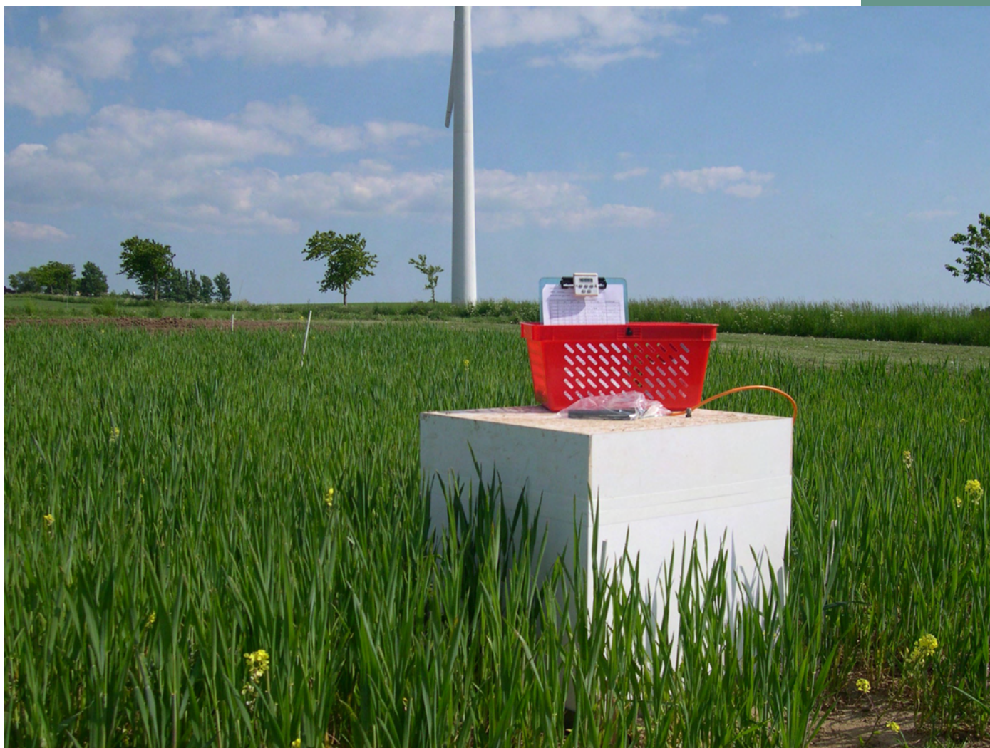
Figure 2: Chamber used to measure N_2O fluxes in the winter wheat crop
