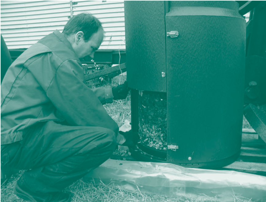
Partial deloading of the compost mass can be possible e.g. by taking off part of the wall.
