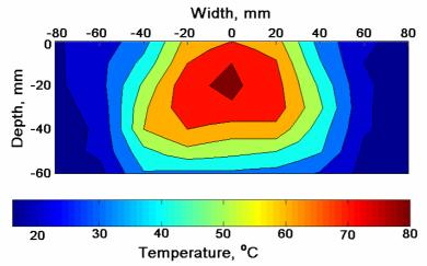
Figure 1. Soil temperatures from a cross-section across the groove, measured 40 sec. after treatment. The width is measured from centre of the treated band. Treated area: With -30 - +30, depth 0 -50 mm.
