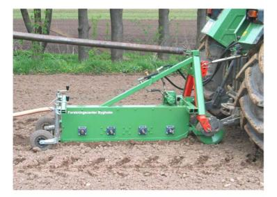
**Figure 3.** Prototype band steaming machine
