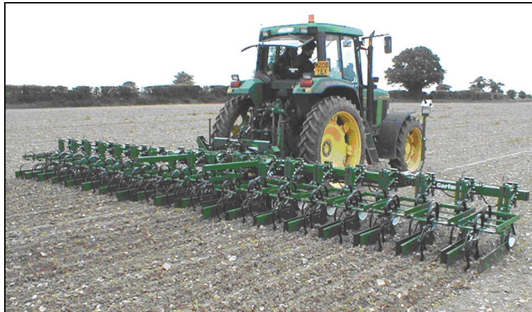
Plate 1. Inter-row hoeing using crop protectors at an early growth stage in sugar beet.
