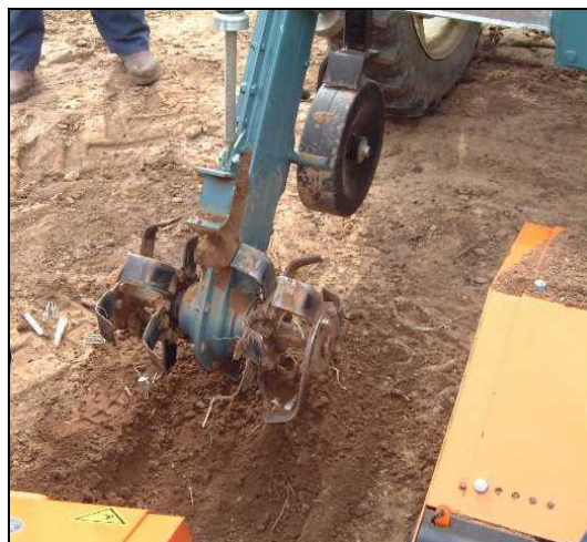
Plate 12. Powered rotary inter-row weeder
