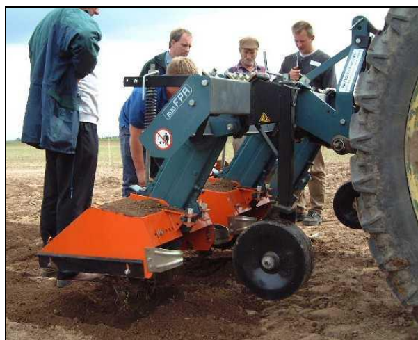
Plate 12. Powered rotary inter-row weeder
