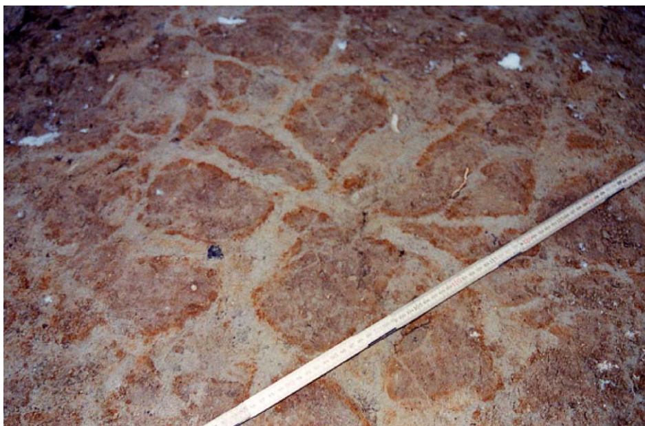
Fig. 2. Photo showing bleaching and Fe(III) enriched rims along fractures at 1.7 m depth from the forest site (see Jørgensen and Fredericia, 1992, for mineralogical explanation).
