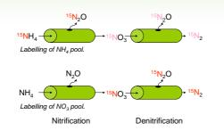
Principles of <sup>15</sup>N isotopic labelling approach used in this study. The fractional contribution of nitrification and denitrification to N<sub>2</sub>O emissions is assessed by comparison with enrichments of the  $NH_{4^-}$  and  $NO_{3^-}$  pools (data not presented).
