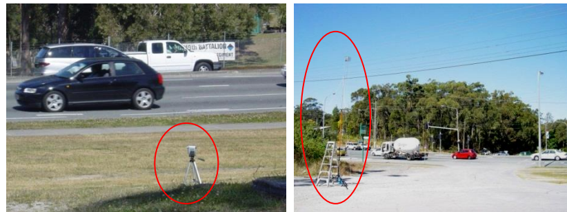
Figure 17: Nerang data camcorder recording signal timing and traffic flow
