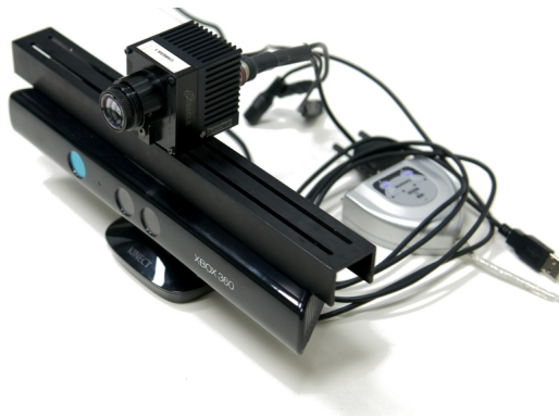
Fig. 2: The sensor configuration prototype: comprised of a Microsoft Kinect and Thermoteknix Miricle 307K thermal camera.
