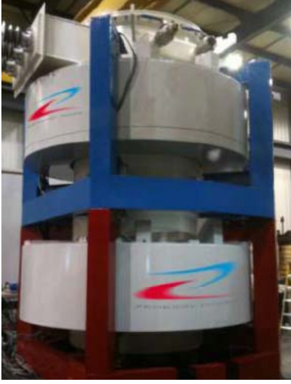
Figure 3 HTS FCL Full scale prototype for 11kV application
