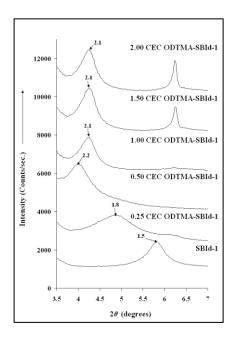
Fig.1. XRD pattern of beidellite and organo-beidellite.
