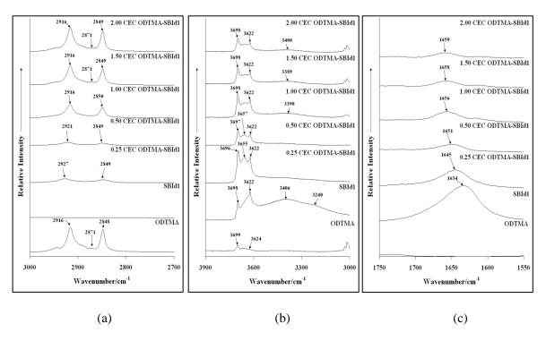
**Fig. 2.** (a) IR spectrum showing C-H stretching region of beidellite and organo-beidellite, (b) HOH stretching region, (c) Hydroxy bending region
