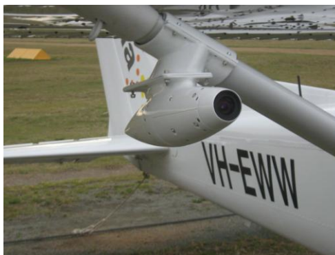
Fig. 3: Camera pod mounted on wing strut of Cessna 172 ownship (chase aircraft).
