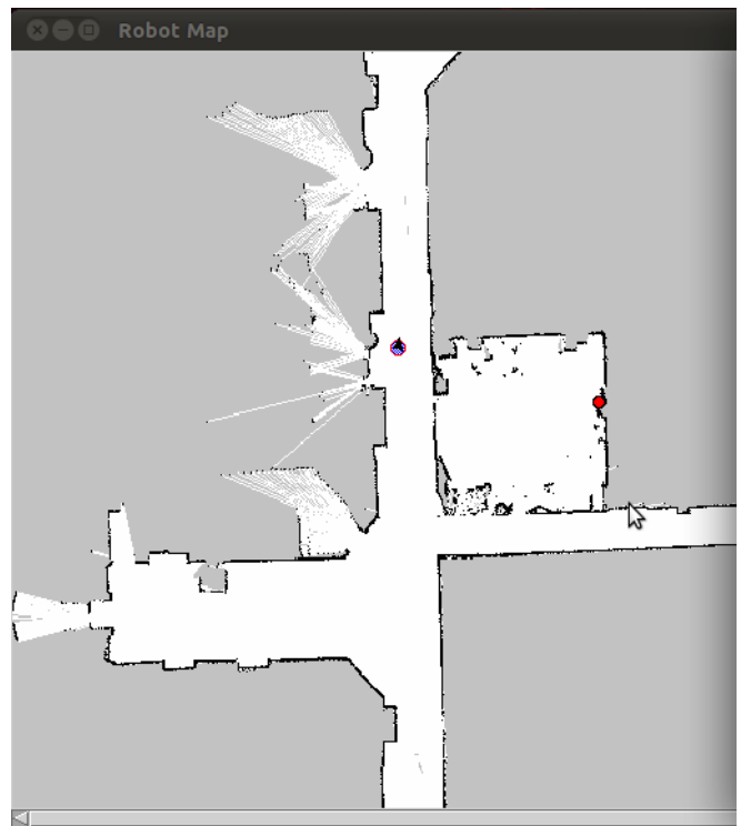
Fig. 5. Remote map view for map-based navigation. The robot’s current pose is shown as a circle with a direction indicator (shown in the middle of the long vertical corridor). The red dot to the right is the origin of the robot’s map.
