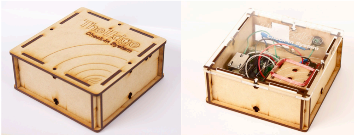
Figure 3: The design for the for the checkin-points is based on digital fabrication methods such as CAD and laser-cutting, and can be easily and cheaply reproduced by any library using local facilities.
