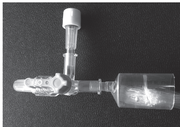
Figure 2. Fiber bundle header and inlet valve. Medium and cells are injected into the system through the syringe port, thus facilitating sterile fluid exchange. Following cell loading the three-way valve was used to isolate the fiber bundle and thus to prevent axial medium movement over the duration of the culture.
