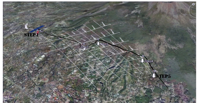
Fig. 1. A planned path that exploits wind energy from the start point (step1) to the target point (step5). While Step 2, Step 3 and Step 4 are the locations where the UAS changes the heading angle to follow the prescribed path.
