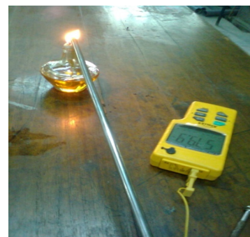
Figure 9: Measurement of different flame temperature by Digital Pyrometer.
