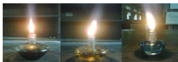
Figure 8: Flame of Mahogany seed oil, Diesel fuel & kerosene fuel
