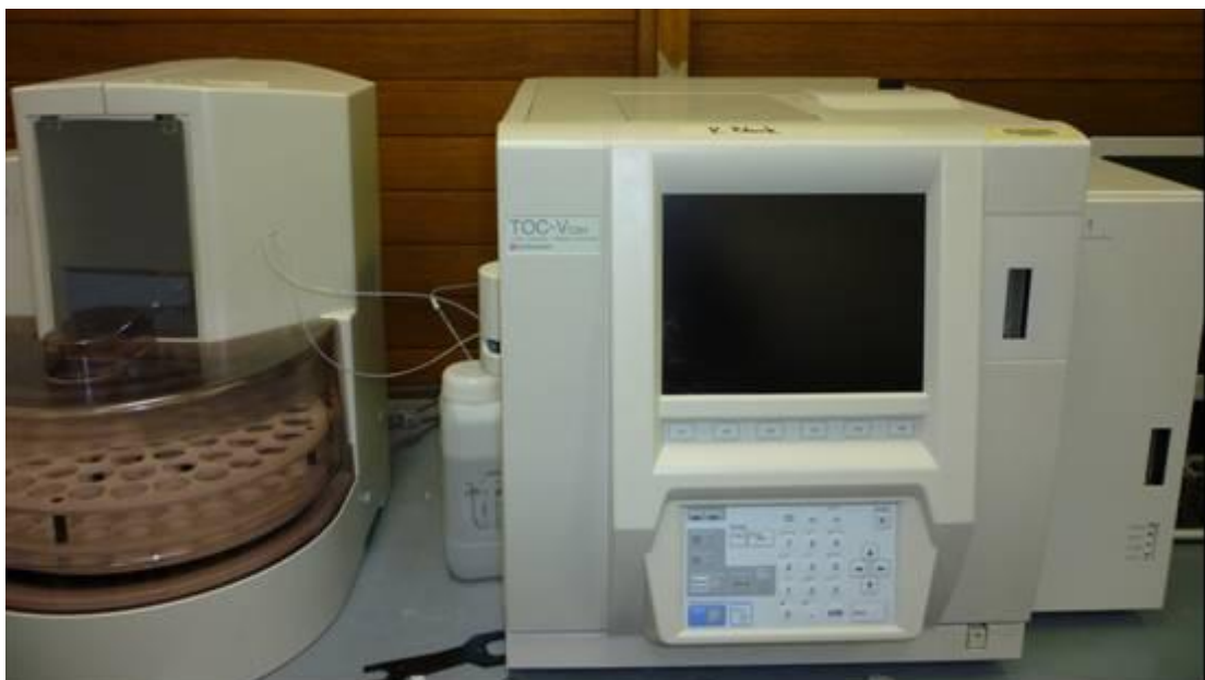
Figure 5-10: Shimadzu TOC-VCSH Total Organic Carbon Analyser
