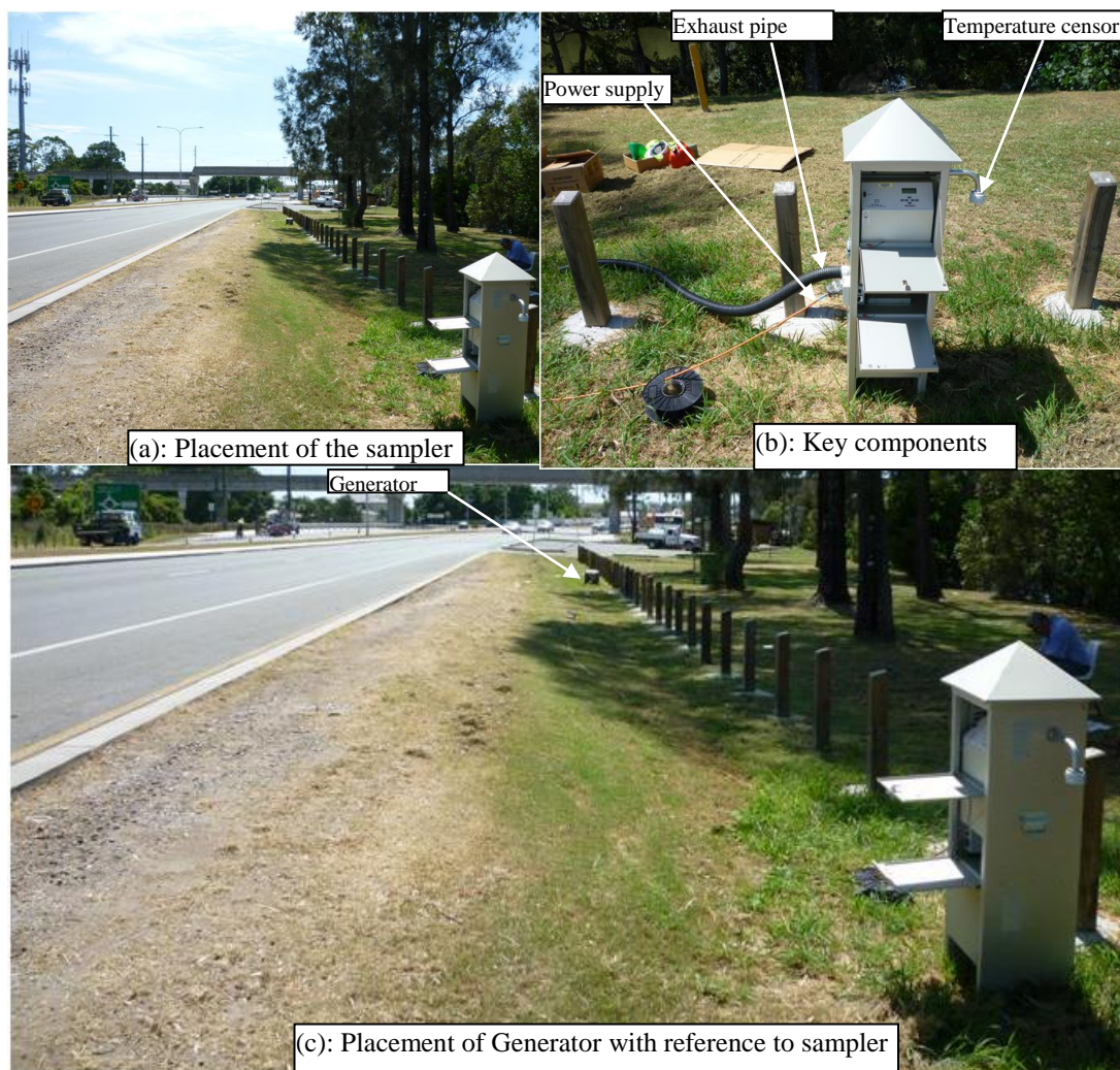
Figure 5-2: Air sampling, (a): placement of the sampler, (b): key components, (c): placement of generator with reference to sampler
