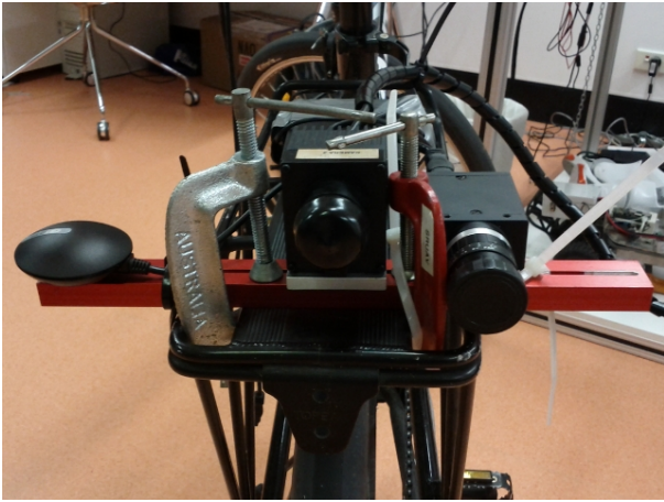
Fig. 2. Capture platform, with (from left to right) the GPS receiver, thermal-infrared camera and visible-spectrum camera.
