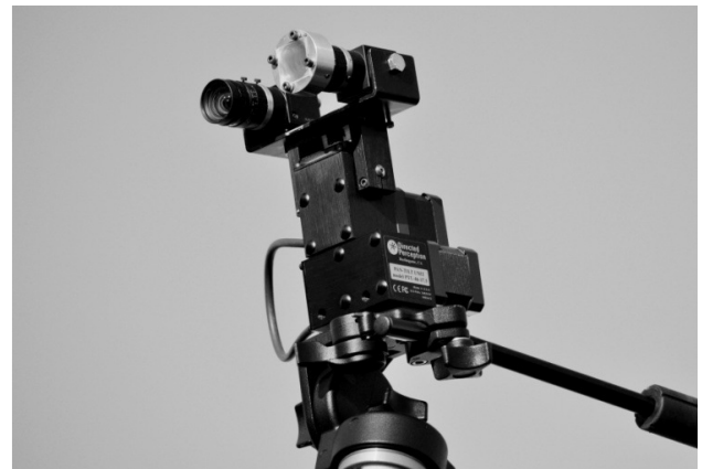
Fig. 1. PTU and camera equipment used for the Hayabusa re-entry
