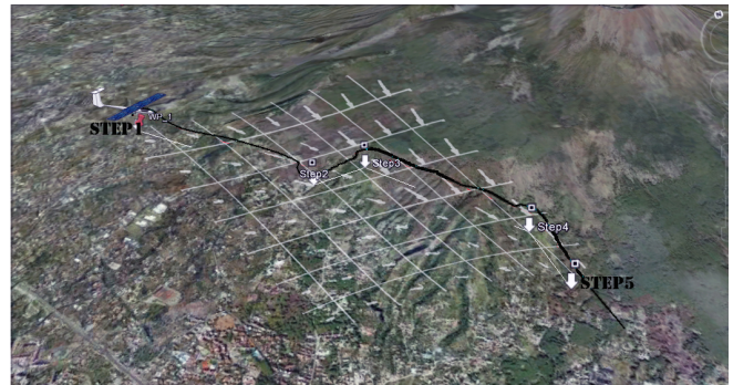
Fig. 1. A planned path that exploits wind energy from the start point (step1) to the target point (step5).
