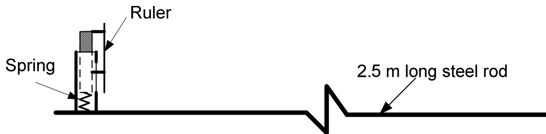
Figure 16: The device used in the pipe to measure its deflection
