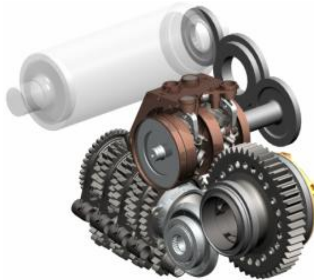
Figure 3-3 Concept diagram for a kinetic energy recovery system (Gizmag, 2007)
