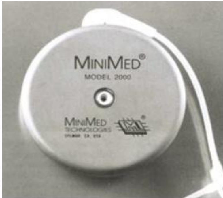
Figure 3-1 The PIMS implantable pump and catheter (NASA, 2009)
