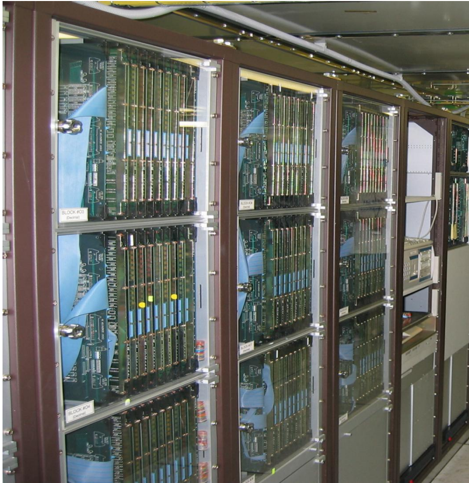
Figure 3-6 Hardware version of correlators at the ATNF, Narrabri, NSW, Australia
